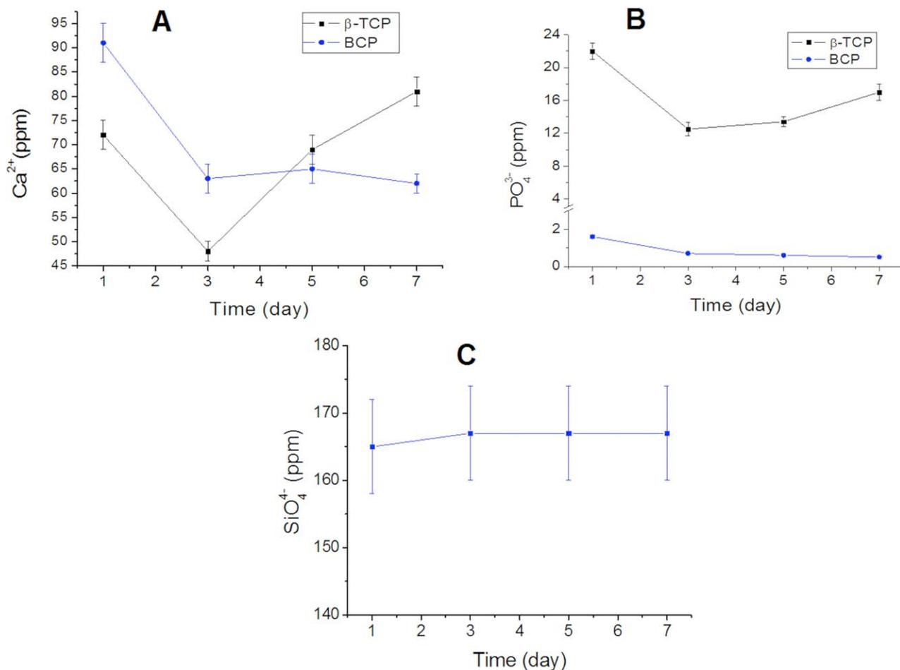
**FIGURE 5.**  $\text{Ca}^{2+}$ ,  $\text{SiO}_4^{4-}$  and  $\text{PO}_4^{3-}$  release from  $\beta$ -TCP and BCP ceramics to DMEM during 7 days of incubation. [Color figure can be viewed in the online issue, which is available at [wileyonlinelibrary.com](http://wileyonlinelibrary.com).]
