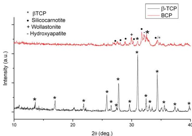
**FIGURE 1.** X-ray diffraction patterns of  $\beta$ -TCP (lower panel) and BCP (upper panel) ceramics. [Color figure can be viewed in the online issue, which is available at [wileyonlinelibrary.com](http://wileyonlinelibrary.com).]
