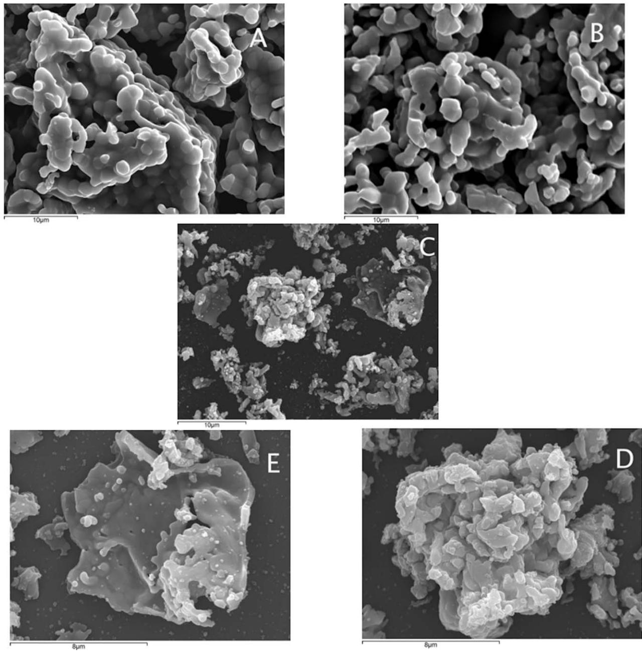
FIGURE 2. SEM images of the undoped  $\beta$ -TCP ceramic (A and B) and BCP (C,D and E).
